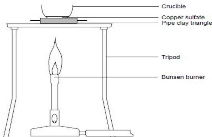
**c** Heat the crucible and contents, gently at first, over a medium Bunsen flame, so that the water of crystallisation is driven off steadily. The blue colour of the hydrated compound should gradually fade to the greyish-white of anhydrous copper (II) sulphate. Avoid over-heating, which may cause further decomposition, and stop heating immediately if the colour starts to blacken. If over-heated, toxic or corrosive fumes may be evolved. A total heating time of about 10 minutes should be enough.
